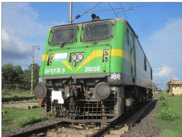
WAG-9 class 3-phase freight locomotive (31000 to 31021 imported from ABB)
