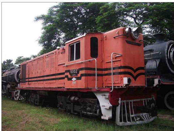
North British Locomotive built YDM-1 class locomotive
