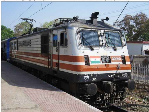
3-phase Bo-Bo type light passenger locomotive class WAP-5 (30000 to 30010 imported from ABB)
