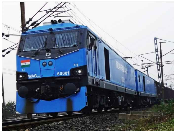
A 12000 hp dual unit WAG-12B class freight locomotive
