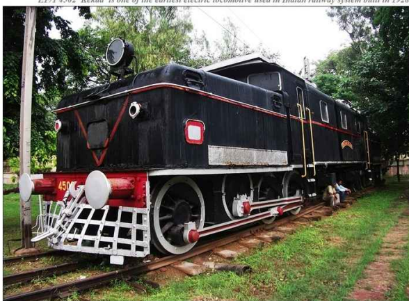
EF/1 4502 'Kekda' is one of the earliest electric locomotive used in Indian railway system built in 1928
