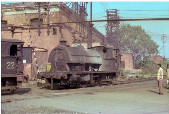
UK built Robert Stephenson and Hawthorn 0-4-0 saddle tank at Kulti pipe factory
