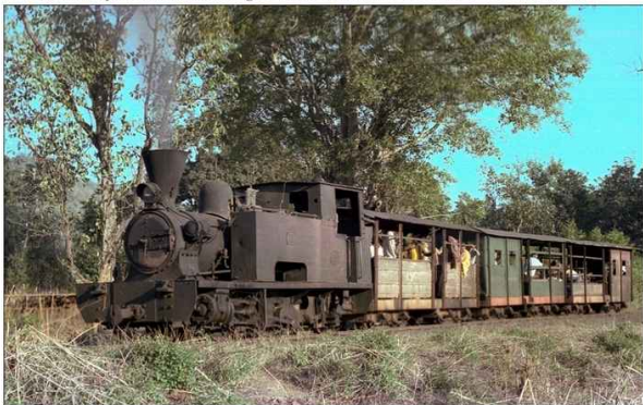
Andrew Barclay built 0-4-2 tank engine No 28 on the line to Chiria with a mixed load.
