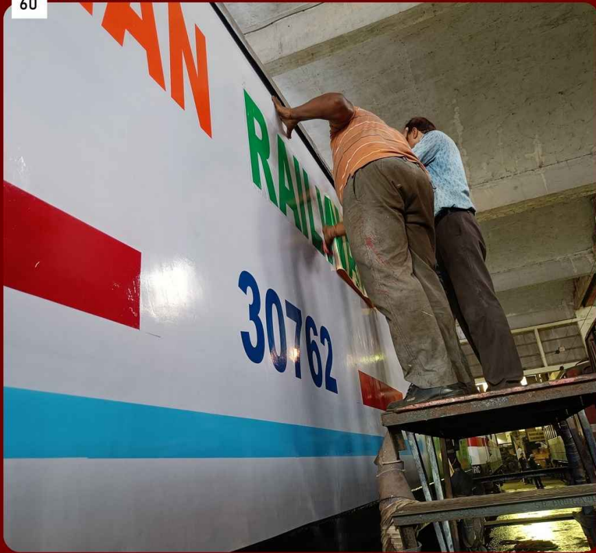
Side profile stencilling going on at Santragachi ELS.
